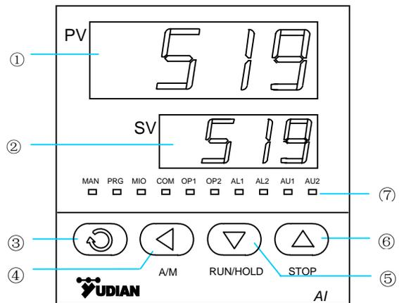
The lighting of MAN means in manual output status. MIO, OP1, OP2, AL1, AL2, AU1 and AU2 indicate I/O operation of the corresponding module. For example, That the COMM indicator is lighting means that the instrument is communicating with computer.
