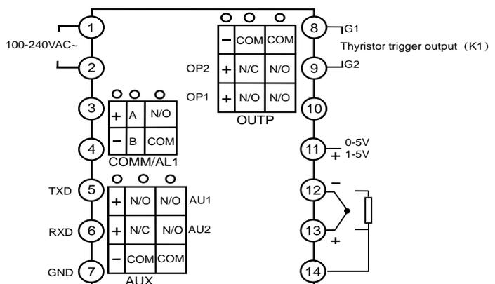
module is installed in COMM and parameter "bAud" is set to 1, then on-off signal can be inputted, and SV1 and SV2 can be switched by connecting a switch between terminals 3 and 4.
