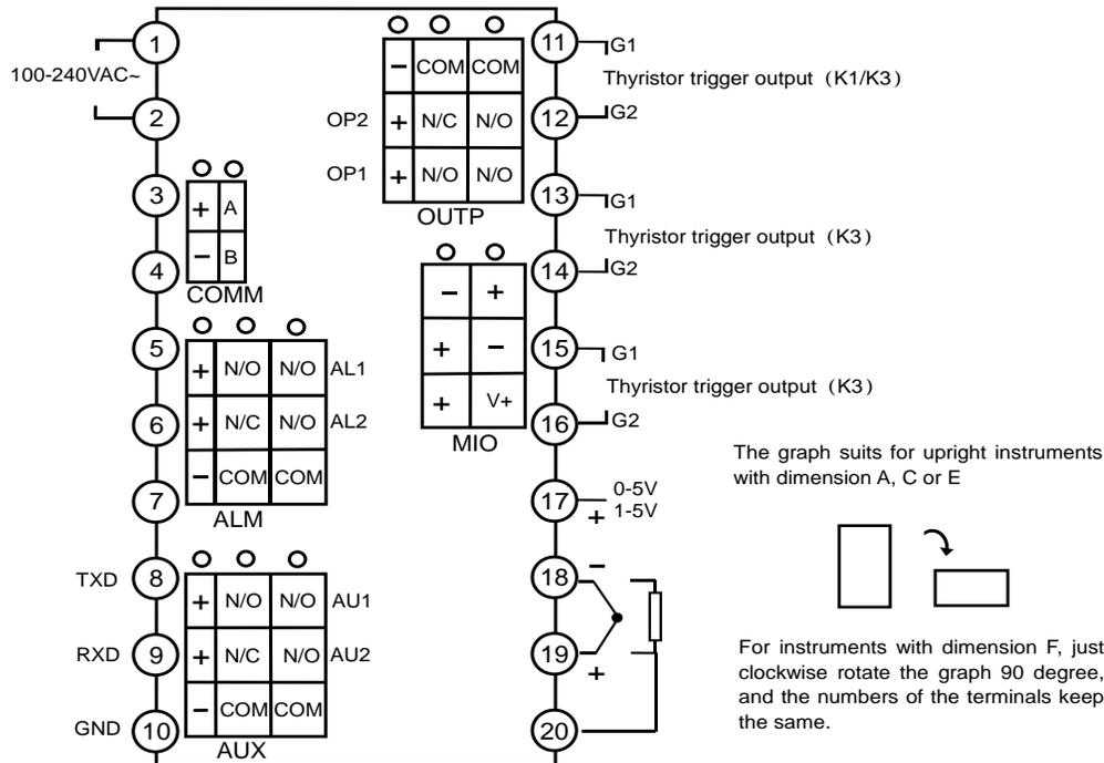
Note 1: For linear voltage input, if the range is below 1V, connect to terminals 19 and 18. 0~5V or 1~5V signal can be inputted from terminals 17 and 18.
