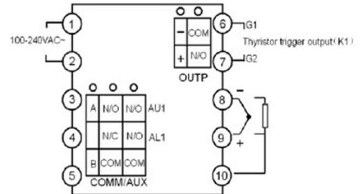
**Wiring graph of thyristor trigger output is as below (suitable for module K1, K3, K5 and K6):**
