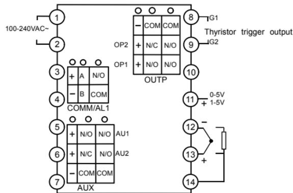
**Wiring graph of instruments with D2 dimension as below:**
