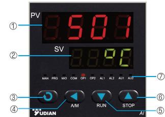
**Basal display status :** When power on, the upper display window of the instrument shows the process value (PV). This status is called basal display status. When the input signal is out of the measurable range (for example, the thermocouple or RTD circuit is break, or input specification sets wrong), the upper display window will alternately display “orAL” and the high limit or the low limit of PV.
