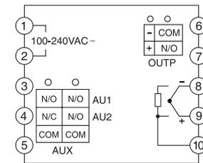
Note 1: Thermocouple should be directly connected to the back of the instrument wiring screws by compensation wires. No conventional conducting wires should be used in the input circuit. Pay attention to the correct type of compensation wires and polarity.
