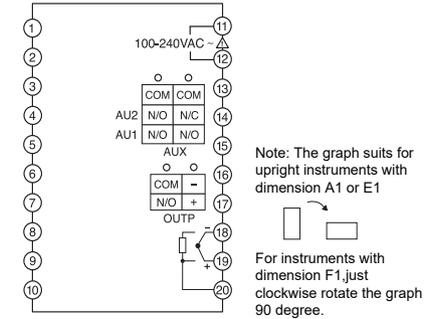
Wiring graph for dimension D (72X72mm)instruments:
