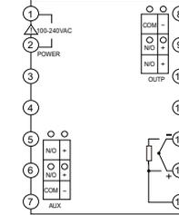
Wiring graph for dimension D21 (48X48mm)instruments:
