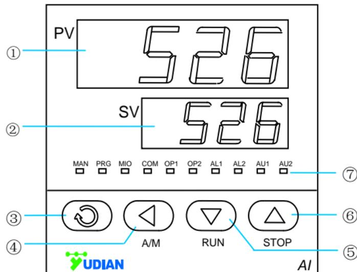
**Basic display status** : When power on, the upper display window of the instrument shows the process value (PV), and the lower window shows the set point (SV). This status is called basic display status. Symbol description was shown as following table:
