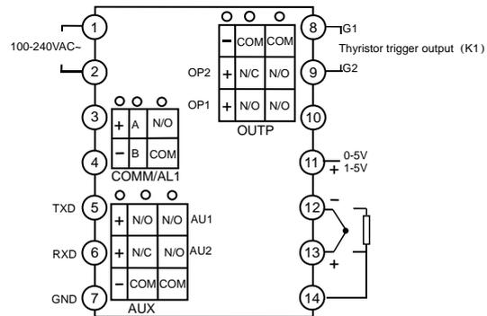
Note 2: 4~20mA linear current signal can be converted to 1~5V voltage signal by connecting a 250 ohm resistor and inputted from terminals 11 and 12.
