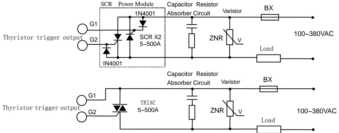
Note 1: According to the voltage and current of load, choose suitable varistor to protect the thyristor. Capacitor resistor absorber is needed for inductance load or phase-shift trigger output.
