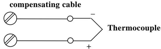
**(1) Internal automatic compensation connected**
