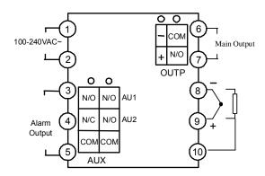
Wiring graph for D dimension (72mmX<u>72mm</u>) instruments
