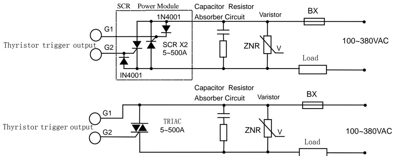
Note 1: According to the voltage and current of load, choose suitable varistor to protect the thyristor. Capacitor resistor absorber is needed for inductance load or phase-shift trigger output.
