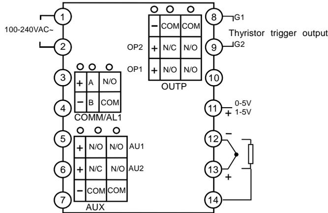
Note 1: Linear voltage signal of range below 500mV should be inputted from terminals 13 and 12, and signal of 0~5V and 1~5V should be inputted from terminals 11 and 12.
