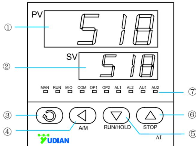
**Basic display status** : When power on, the upper display window of the instrument shows the process value (PV), and the lower window shows the set point (SV). This status is called basic display status. Symbol description was shown as following table:
