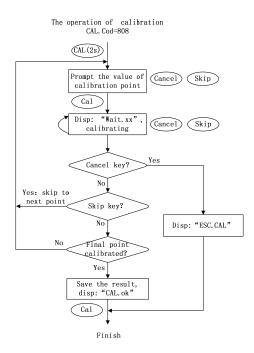
(4) Calibration for Errors of the Interior Reference Ends: Set CAL.Cod=808, and press "Key 2 + Key 4" for long to enter calibration. Place the instrument in the environment with stable temperature, set the type to the thermocouple with larger thermoelectric potentials (K thermocouple or E thermocouple is favorable and B thermocouple, S thermocouple or R thermocouple is not suitable), set
