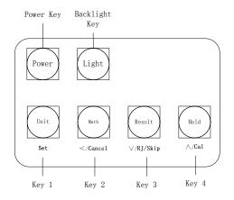
Keys are divided into three types including the short keys, long keys and combination keys. Long keys or key combinations (keys should be pressed and hold for 2 seconds) are used to realize the functions of Set, Cancel, RJ or Cal, and short keys are used to realize other functions.
