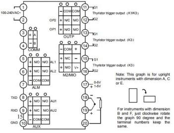
kinds of thermocouple are different, and should be directly connect to the terminals. When the internal auto compensation mode is used, connecting the common wire between the compensation wire and the terminals will cause measurement error.
