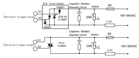
Note 1: According to the voltage and current of load, choose suitable varistor to prevent the thyristor. Capacitor resistor absorber is needed for inductance load or phase-shift trigger output.
