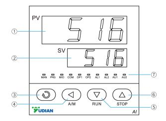
When power is on, the upper display shows the process value (PV) and the lower display shows the set point (SV). At certain circumstances, the lower display blinks SV and the following status message. The symbol message:
