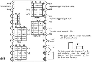
(4) When main output is selected linear current or SSR voltage, the output will be given from terminal 13+, 11-.
