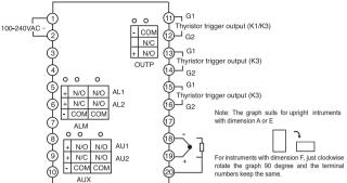
Wiring graph for D dimension(72mmX72m) instruments:
