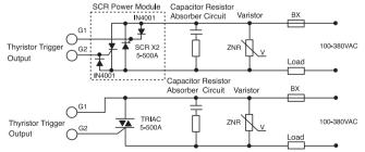
Note: it is recommended to use the SCR power module, which includes a pair of SCRs and diodes. Compared to TRIAC, it is more reliable and consumes less electricity.
