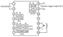
Wiring graph for D2 dimensio (48mmX48mm) instruments
