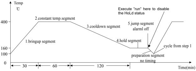
The advantage of applying "temperature-time-temperature" arrangement is to provide a wide window of setting rate of increasing and decreasing temperature. The format of increasing and decreasing temperature steps keep the same format, for ease to learn. There is a high flexibly to set the curve, enabling possibility to input continuous increasing curves (e.g. using different rate of increasing curve to achieve functional heating) or continuous temperature holding steps
