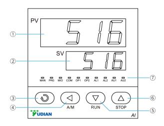
When power is on, the upper display shows the process value (PV) and the lower display shows the set point (SV). At certain circumstances, the lower display blinks SV and the following status message. The symbol message:
